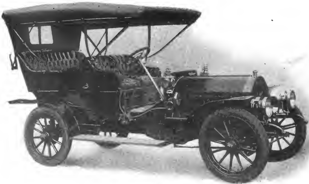
JACKSON TOURING CAR, MODEL E, 4 CYLINDERS, 35-H.P., PRICE $2,000. Jackson Automobile Co., Jackson, Mich.
